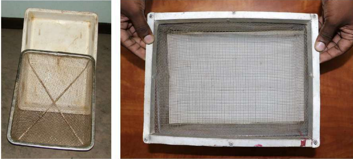
Plate 7 Hand-held litter sifter and the white tray for extracting ants in the leaf litter
