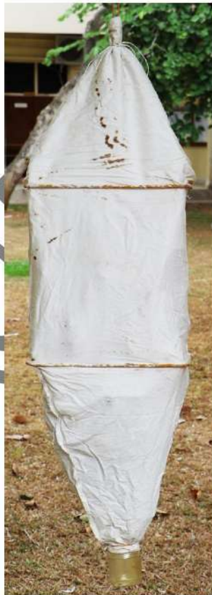
Plate 8 Showing a mini-Winkler bag, which is used to collect ants in the leaf litter
